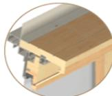
One-piece, full 4<sup>9</sup>/<sub>16</sub>" head and side jamb with inside stop blind nailed to reduce the number of visible nail holes
